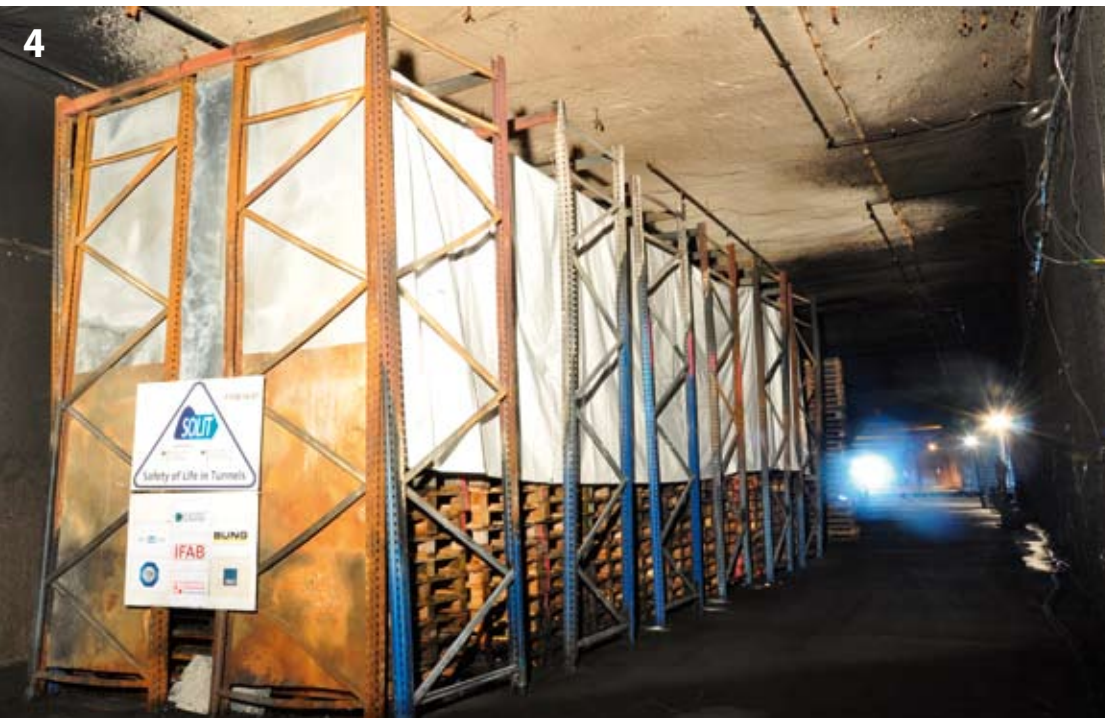
Tarpaulin – covered HGV (truck) fire mock-up [13]
