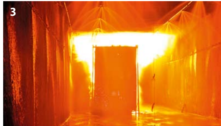
HGV (truck) fire prior to activation of water mist system [2]
