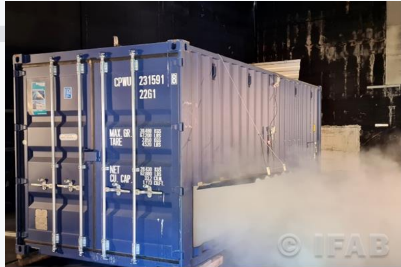
Exhaust gases vented through explosion prevention openings (EPO) during fire test with high-pressure water mist
