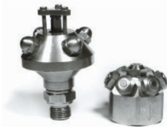
Electrolux Euroclean (HTC) automatic nozzle prototype from 1985 and deluge nozzle from 1983 tests (photo by Håkan Ungerth)
