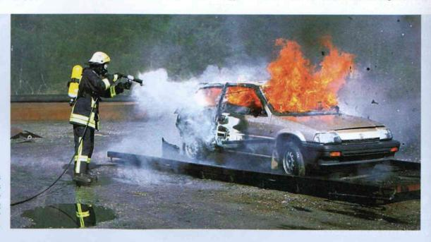
With the Fogtec's Foggun 5, firefighters can choose from five jet settings ranging from pure water mist to a full jet. lessened. This would also be the setting of choice in the final phase of a fire.
