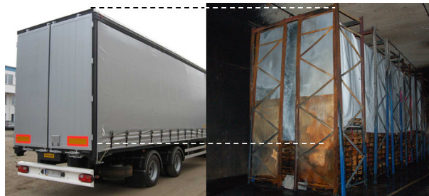
Figure 4. Real trailer and simulating mock-up [31]
